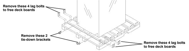
4. Remove the two (2) end deck boards from one end of the pallet and the attached, notched section of the center runners (refer to **Figure 3**).
